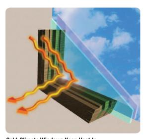
**Cold-Climate Windows Keep Heat In**Double-pane windows with low-e coating on the glass reflect
